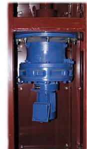
Sumitomo Cyclo Gearbox NO BELTS TO BURN!!
